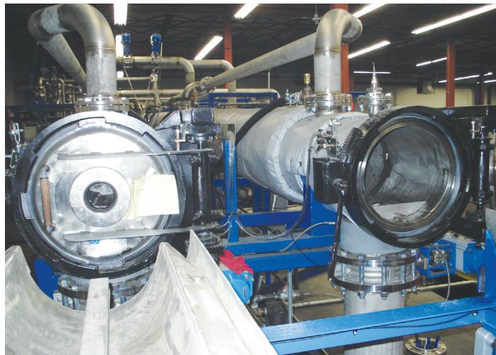
**A tube cleaning vacuum system provides an effective and environmentally friendly alternative to an open dip tank.**
