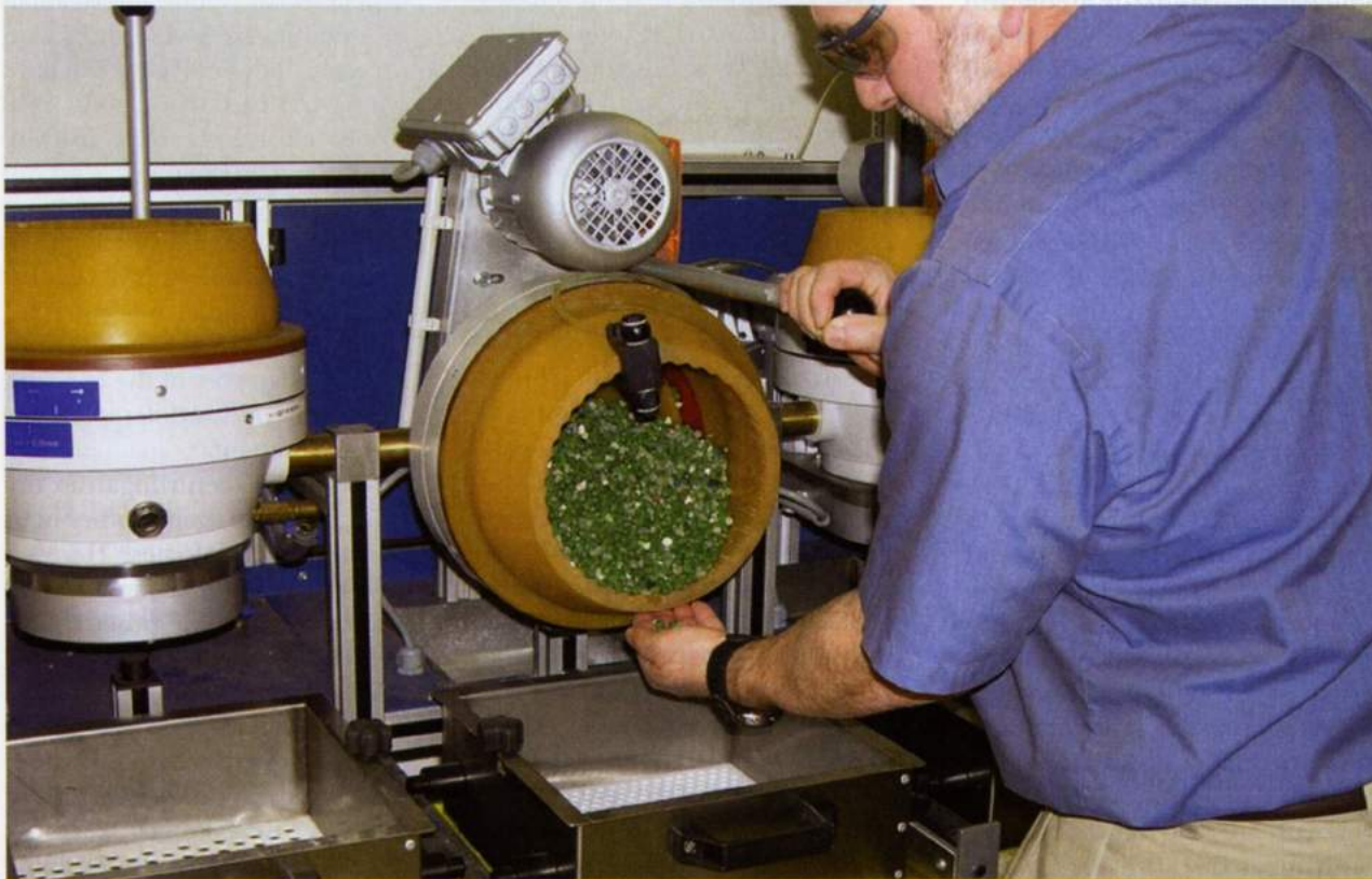
The open process facilitates operator access and allows a continuous flow of water and compound, keeping both media and parts clean.
