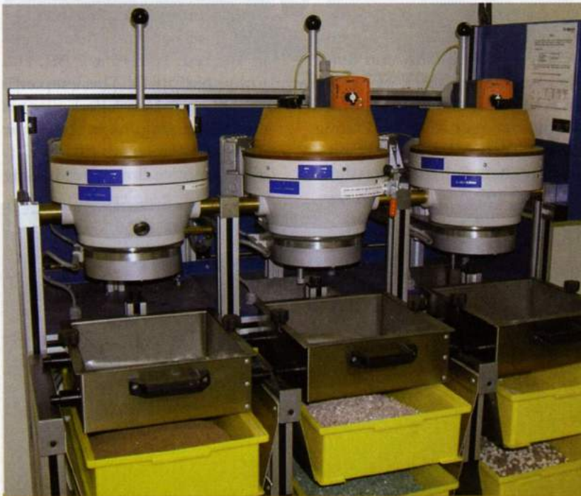
Modular construction lets users easily configure deburring cells consisting of multiple process chambers of a variety sizes. Cells can be set up for deburring, polishing or both.
