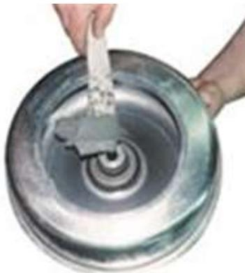
Captured fines collect as sludge in the bowl of the centrifuge system. These fines can be landfilled as non-hazardous waste.
