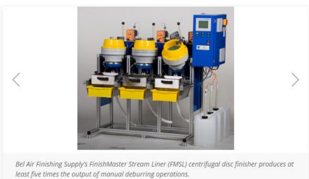
Bel Air Finishing Supply Inc. (North Kingston, RI) centrifugal disc finishers help manufacturers increase throughput, decrease cost, and increase part quality by polishing and deburring a wide range of materials including aluminum, brass, copper, kovar, stainless steel, steel, and titanium. In addition to eliminating 80% of the handwork involved in manual deburring operations, they drastically reduce surface roughness (Ra) of parts for the aerospace, automotive, medical, and other industries.
